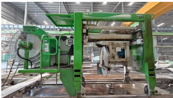
Figure 12: Cutters to cut slabs to desired size
