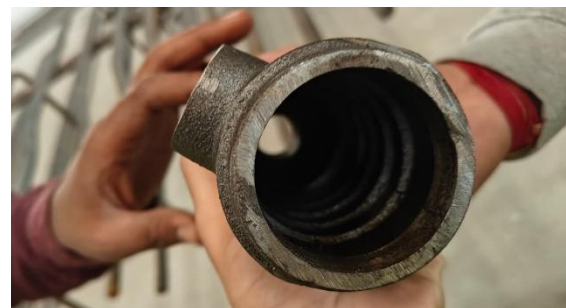
Figure 4b: Hole to insert rebar
