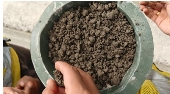
Figure 11: Concrete mix with w/c ratio 0.18
