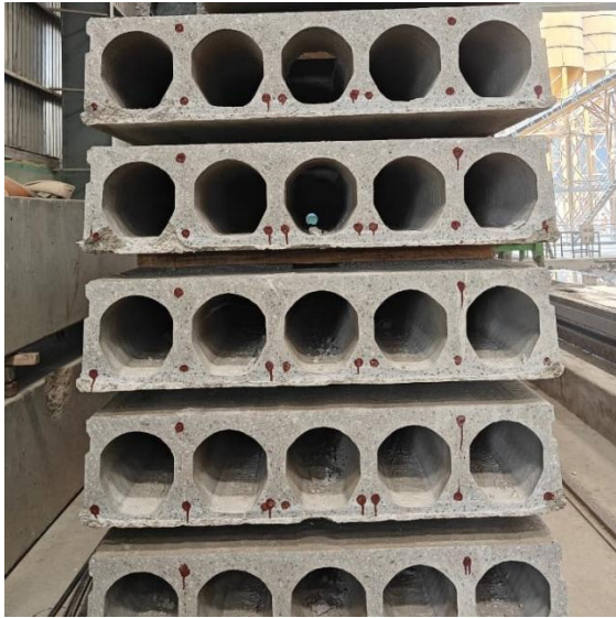
Figure 8: Hollow Core Slabs
