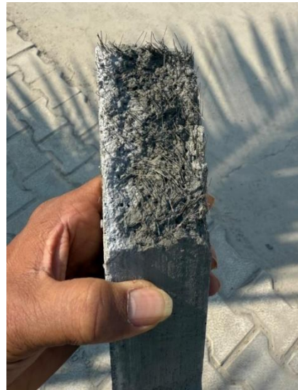
Figure 3b: Fibre reinforced concrete
