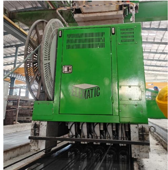
Figure 9: Casting and vibration of hollow core slabs
